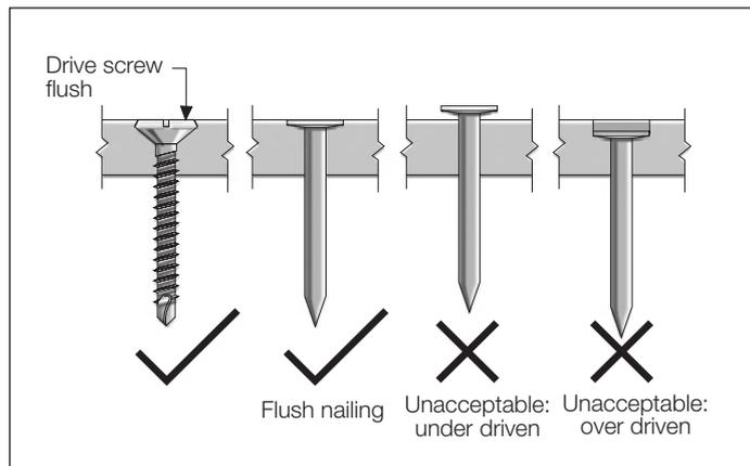
FIGURE 2 FASTENER DEPTH
