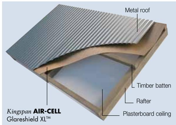
Figure 2 **Kingspan AIR-CELL Glareshield XL™** in a metal roof with a raked ceiling
