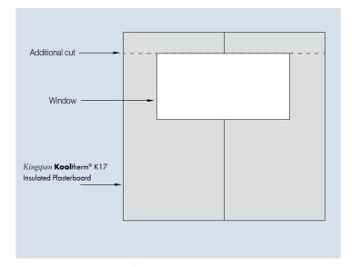
Figure 10  $\it Kingspan$  Kooltherm® K17 Insulated Plasterboard Installation Details for cutting
