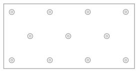
Figure 3 Fastener pattern (11 No. per board)
