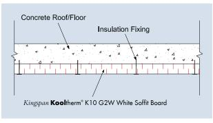
Figure 4 Side elevation - Concrete Soffit with Kingspan Kooltherm $^{\otimes}$  K10 G2W White Soffit Board
